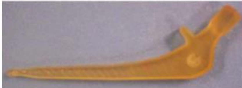
Figure 5.3 Rapid Prototyping (SLA) model of hip prosthesis
